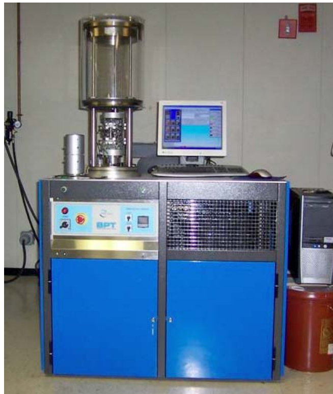
Figure 6-2. Asphalt Mixture Pavement Tester
